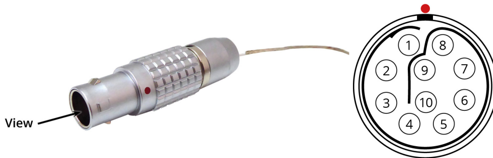
Figure 1.4: Connector Circular, 10 pins, female with viewing direction and pin labelling
