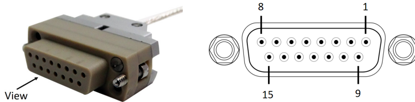
Figure 1.2: Connector D-SUB, 15pins, female with viewing direction and pin labelling
