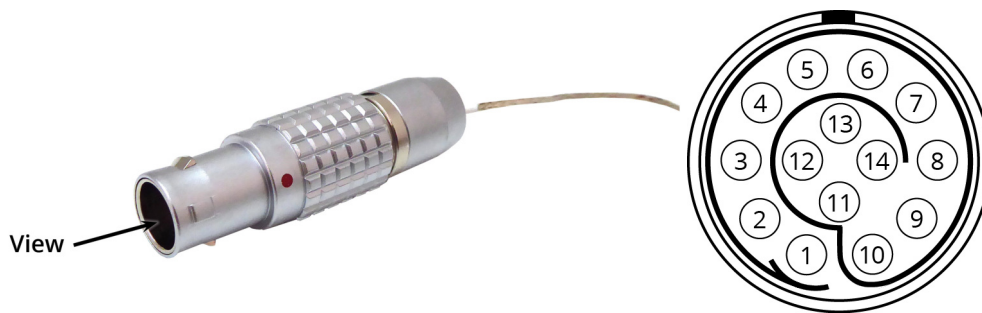
Figure 1.6: Connector Circular, 14 pins, male, UHV with viewing direction and pin labelling
